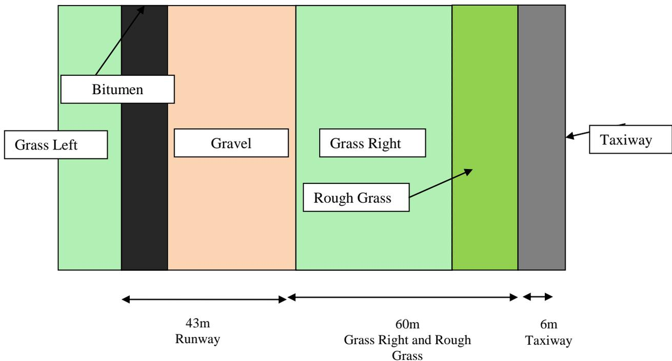
**Note: The above diagram describes Runways 23 and 13. The sequence left to right of the components for Runways 05 and 31 is the reverse of the above diagram.**
